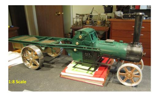
Overall dimensions, 32" long, 12.5" tall, 10" wide, and weighs 25 pounds. Butane fired copper boiler, rest is 303 stainless steel with bronze bearings, cargo deck is wood. Three speed transmission, chain final drive, rear axle has working differential.
